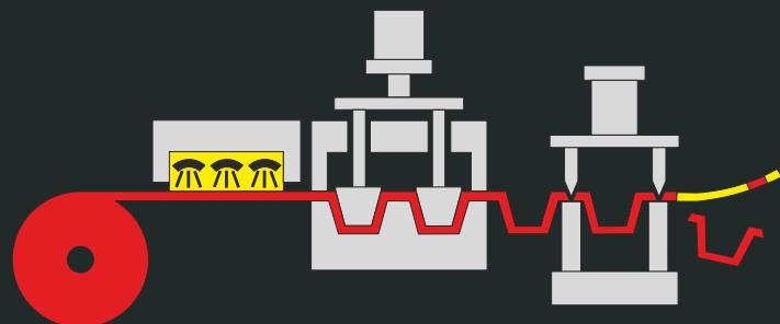
Tools for 3-station Forming - Cutting - Stacking
